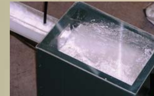
Filter box in laboratory apparatus; suction is applied by a vacuum on the right and foam enters from the left.
