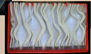
Typical response of full-size FRAM™ air filter to exposure to foam in ingestion experiments.
