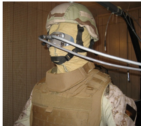
Sweating manikin used in Human Factors work at KSU.
