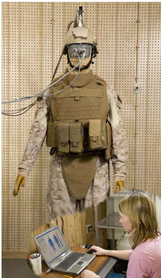
STAN (sweating manikin) tests thermal properties of military uniforms/gear.
